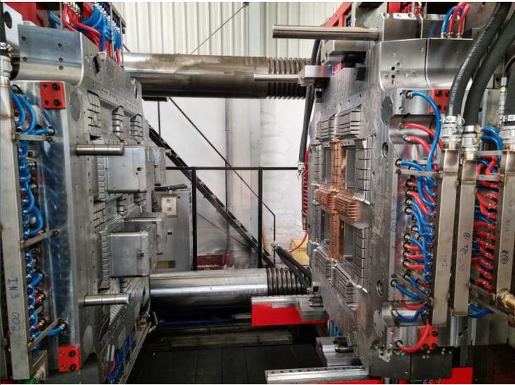
Stack Mould trial for Pallet
